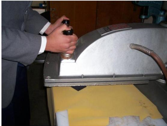
**Photograph .1.2:Cutting in press machine**
